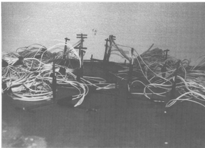
Fig. 2 - Instrumented Three Dimensional Steel Frame Gage
