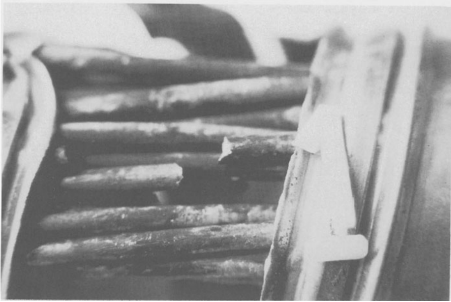
Fig.1 - View of wire failures in fretting-fatigue test.
